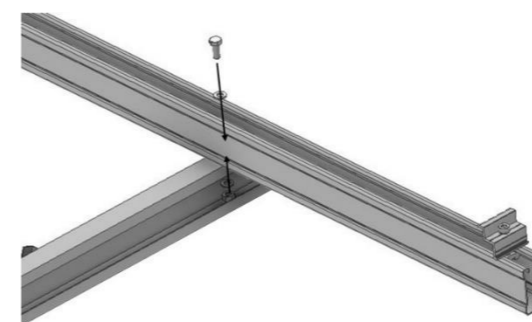
6. RAFTER / PURLIN ASSEMBLY
