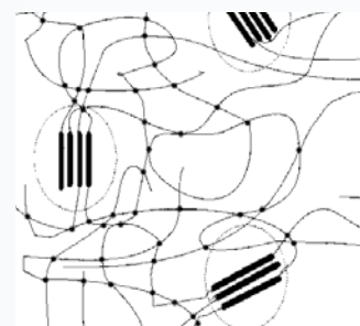
AFTER cross-linking: Schematic representation of chain-forming macromolecules after cross-linking. Three-dimensional cross-linking of polymer chains (heavily impaired freedom of movement).
