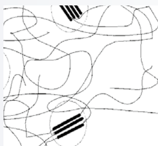
BEFORE cross-linking: Schematic representation of the chain-forming macromolecules before cross-linking. Free movement of polymer chains (in the melt and in the solution).
